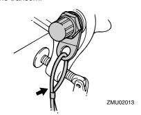
Secure the clamp bracket to the transom using the bolts provided with the outboard (if packed). For details, consult your Yamaha dealer. WARNING! Avoid using bolts, nuts or washers other than those contained in the engine
